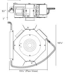
HOUSING: Fabricated of 20 ga. galvanized steel with thru wire J-box, 4 in 4 out at min. 90°C, #12 AWG thru branch circuit wiring. IC-rated housings for use with 14W light engines only are rated for direct contact with spray foam insulation of R-42 per inch or less. IC-rated housings for use with 20W light engines are rated for direct contact with spray foam insulation of R-3.7 per inch or less.
