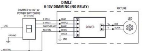
If switched, non-dimming operation is desired, cap off purple and gray wires individually at installation. Do NOT cap purple and gray wires together.
