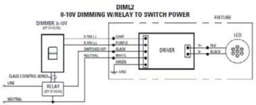
If switched, non-dimming operation is desired, cap off purple and gray wires individually at installation. Bo NOT cap purple and gray wires together.
